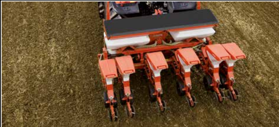
PP1400TE with 6 rows, 4.0m working width telescopic frame, 440l fertiliser hopper
