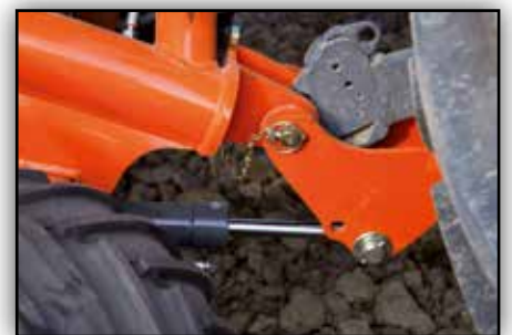
Optional hydr. frame ballasting kit
