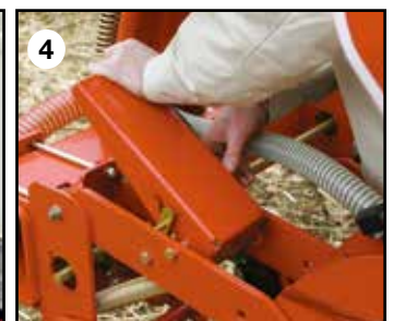
Additional row ballasting
