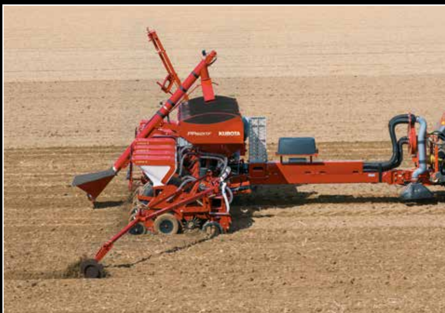
PP1601TF 8 row trailed with fertiliser applicator
