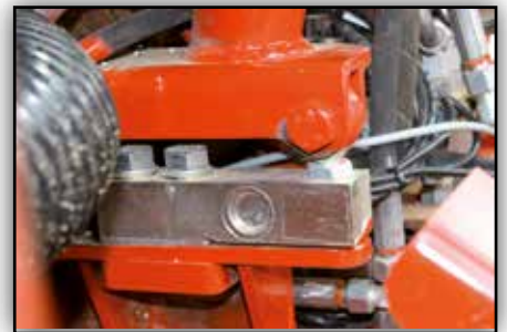
Weigh cells for the precise and controlled fertiliser application
