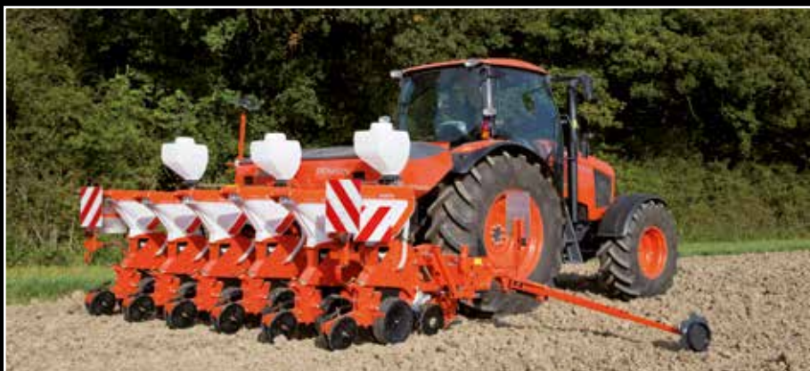
PP1450V e-drive II: 6-row telescopic, 4.5m working width, 1000l fertiliser hopper
