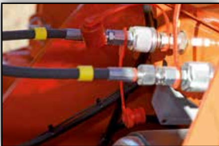
Interface of the hydraulic and electric connections in the headstock of the power harrow
