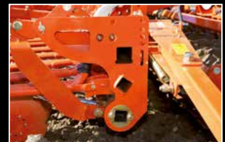
Overload protection of the marker arm
