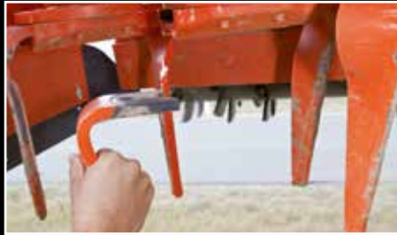
Quick-Fit tines – the tines are locked in position by a pin and clip. Tines are quickly replaced without tools.
