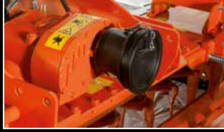
Robust change gear box with replaceable gears as standard. Additional sets of gears are available.
