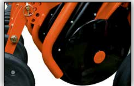
CX-II coulter with double entry for fertiliser application (red tube) and seeding (black tube) in one pass.
