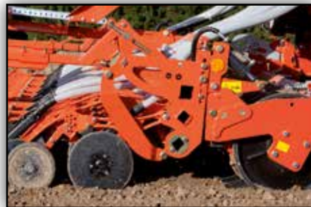
The coulter bar is directly connected to the packer roller frame.
