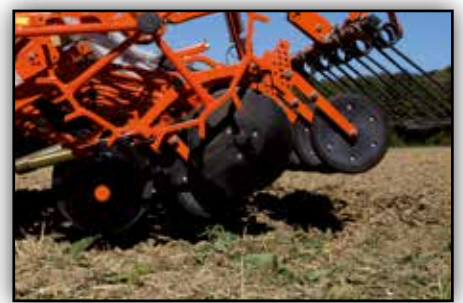
Should the power harrow need to be used solo during sowing, the coulter bar and metering landwheel can be lifted completely via the two integrated hydraulic cylinders of the optional hydraulic coulterbar lift system. This is especially advantageous if furrows are to be closed or if the headland is only to be tilled.
