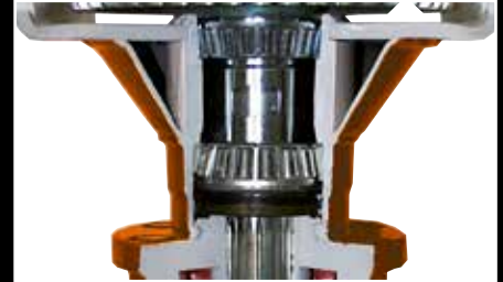
Two large conical bearings with a wide distance provide rigidity and a long service life.
