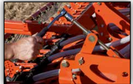
The mechanical coulter pressure adjustment is standard equipment, the hydraulic version is optional
