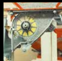
Setting for fine seeds, with rotary brush
